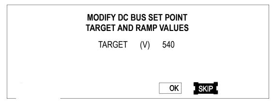
New Target and Ramp settings are temporary settings for diagnostic testing or special situations. Each time the UPS is placed online, the settings return to the default values. Custom T and R entries are only allowed when rotary switch is in Bypass position.
